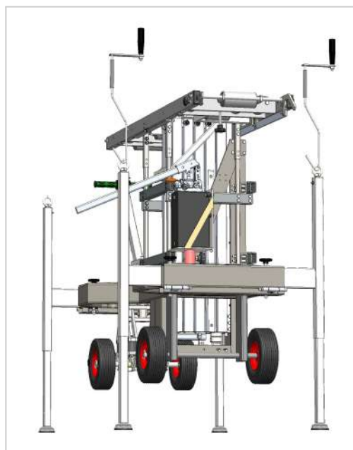
View of the outriggers extended with removable screw cranks
