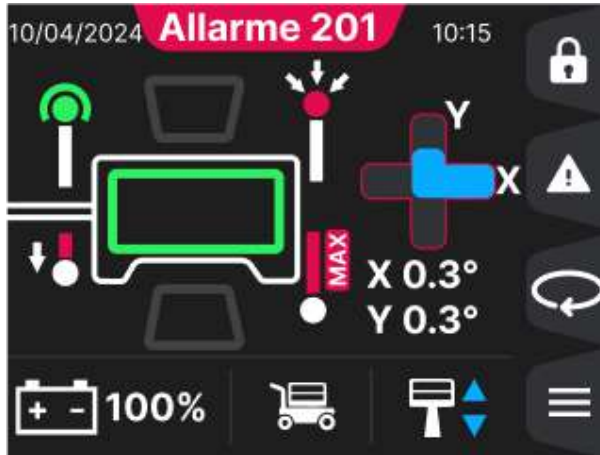
Display – overview in lifting mode (top view)
